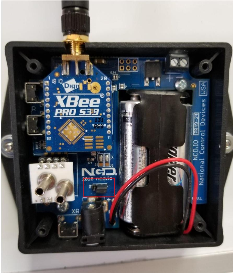
battery mode, open the sensor case and shift the power pin jumper over one. The red rectangle shows the power jumper mentioned and is shown in the battery powered position. Once this is in place, the sensor will automatically connect to the wireless gateway. Depending on the factory settings, it may take 10 minutes or so for the sensor to send
